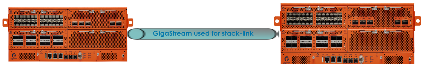
Figure 4 Daisy-Chain Configuration using GigaStream for Stack-link
